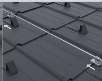
Clip the lightning protection wire into the conductor holder.
