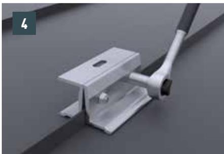
4 The two stainless steel nuts should be tightened to a torque of 35 Nm.
